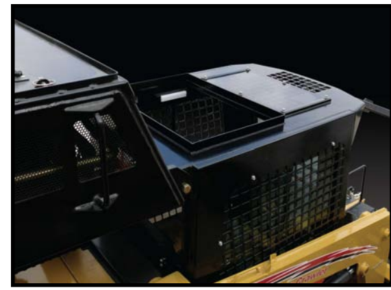
Roof Top Escape Hatch
