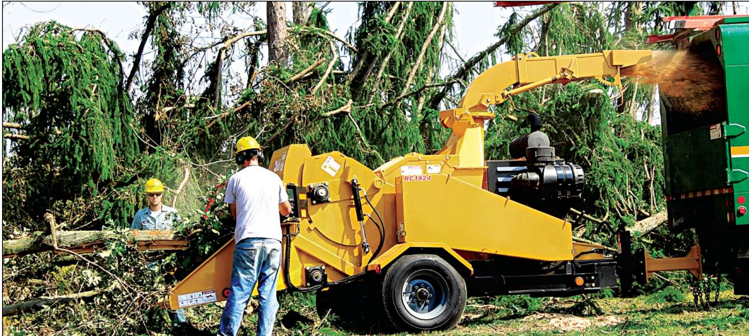
RC1824's powerful feed system pulls in brush, limbs, and logs easier with less trimming.
